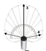
The range, respectively the G-Sonic model is determined by the length 3) of the water object. The click generator has an opening angle of approx. 160° 4), comparable to a underwater music loudspeaker.
